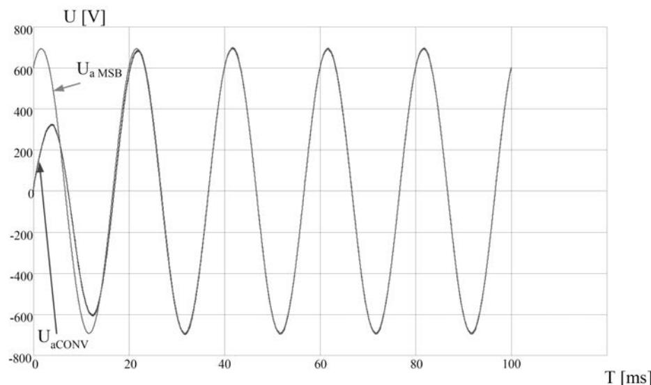
**Fig. 7 Voltage Waveform of Phase "a"  $U_{a\text{MSB}}$  of ship network and Voltage Waveform of Phase "a" of converter STS system  $U_{a\text{CONV}}$  during synchronization with using PLL**
