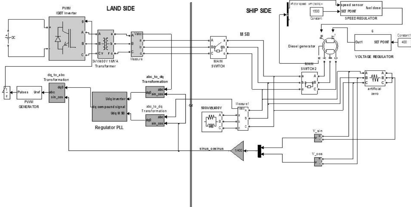
**Fig. 6 The simulation model of synchronization in the STS system employing PLL**
