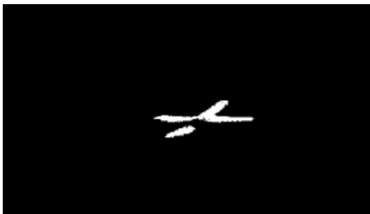
Fig. 18 Binary image of the middle mark after removal of impurities
