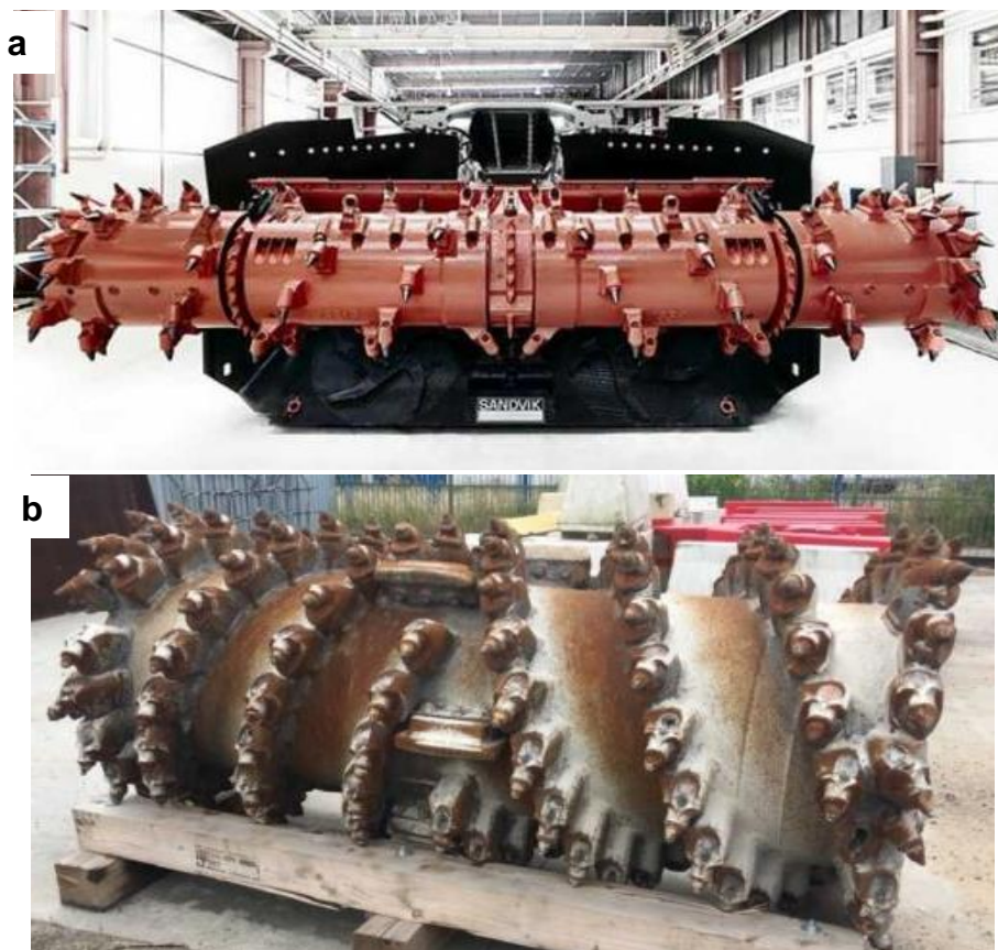
Fig. 5 Cutting drums (a. on the left a Sandvik road header, b. on the right a Wirtgen road milling cutter)
