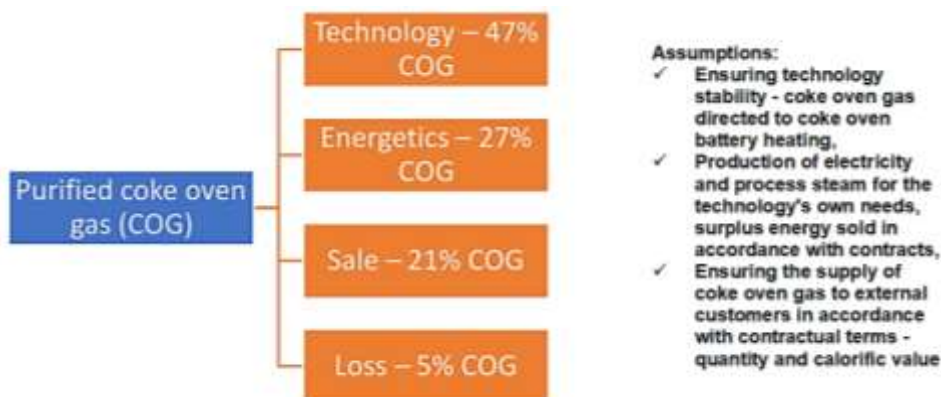
Fig. 1 Utilization of coke oven gas produced in the coking plants of the JSW Group
