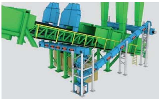
Fig. 5 The system of collecting representative samples simultaneously from two conveyors – intended for high-capacity transport systems
