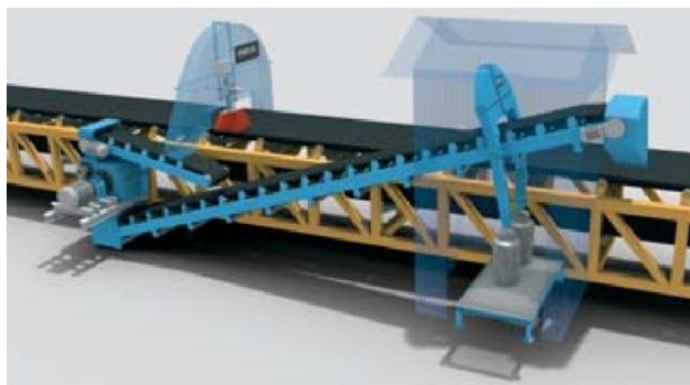
Fig. 4 Sampling system with two samplers and a crusher with a division of the sample into two containers
