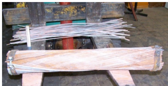
Fig. 1 A section of damaged rope intended for testing
