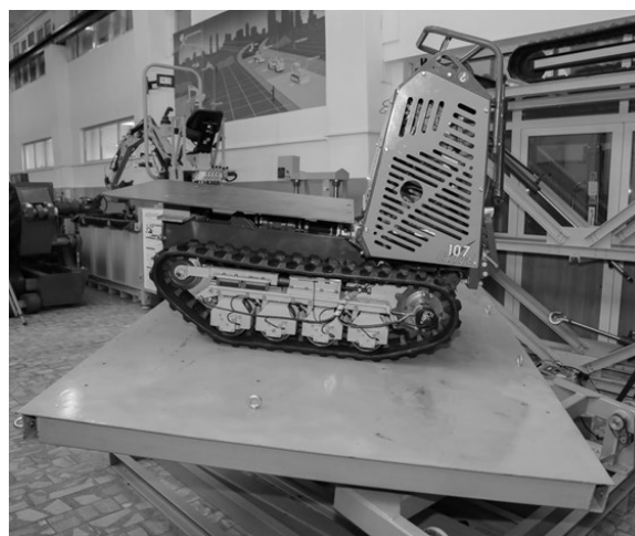
Fig. 7 The vehicle used for tests of the developed system for monitoring of tip-over stability
