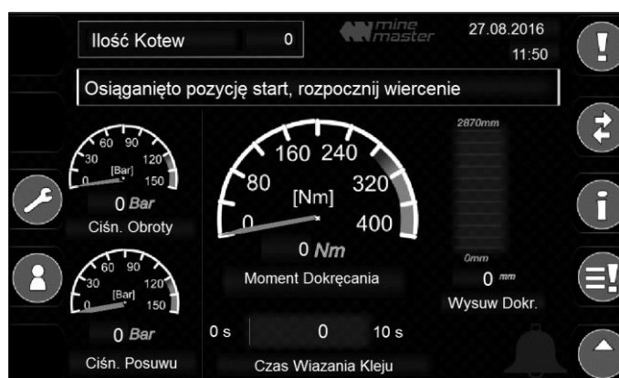
Fig. 2 Bolting installation support system – view of the operator control panel
