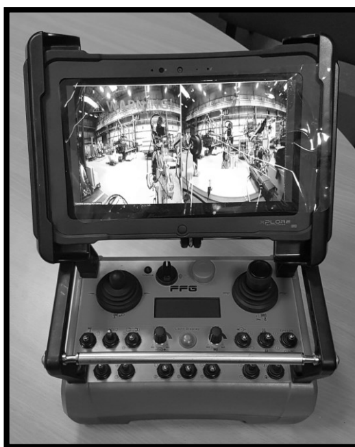
Fig. 3 Drilling rig remote control produced by Cavotec company
