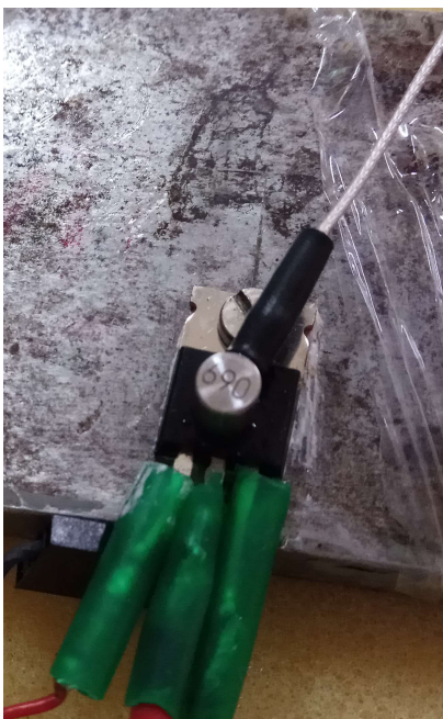
Fig. 3 Transistor with a sensor on a radiator
