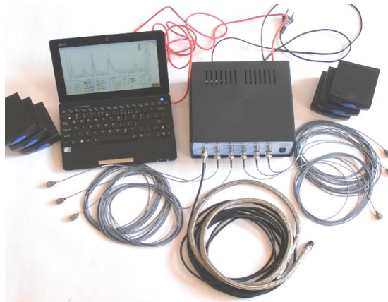
Fig. 3 Submarine internal combustion diesel engine condition monitoring system built in PNA
