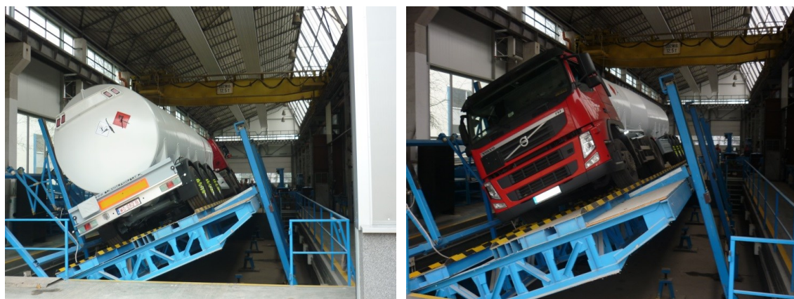
Fig. 1. Test rig (tilt table) for determining the static transverse stability.
