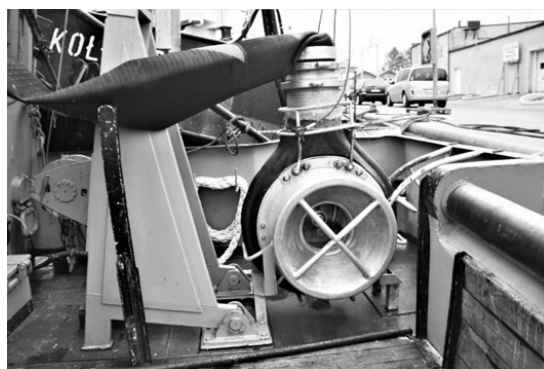
Fig. 4. Impeller pump with hydraulic drive to transfer fish from net to sorting machine.
