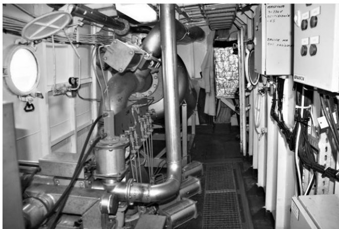
Fig. 5. Vacuum system for fish transport from RSW tanks to tanks onshore.
