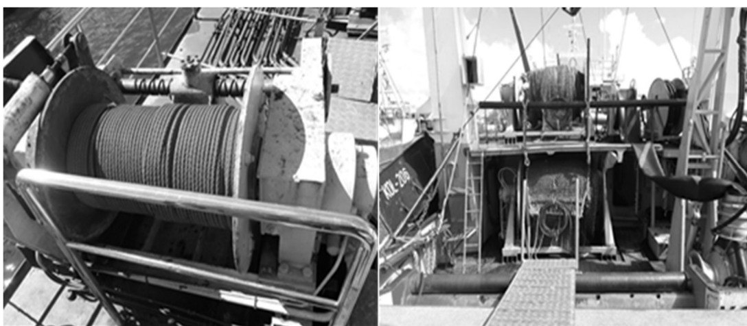
Fig. 4. Trawl winch (on the left) and net winches (on the right) on KOŁ 206.
