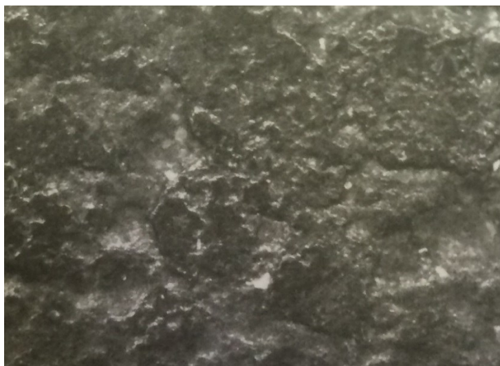
Fig. 4. Microstructure of rubber conveyor belt surface. Exposure in soybean oil for 50 hours and UV for 100 hours.
