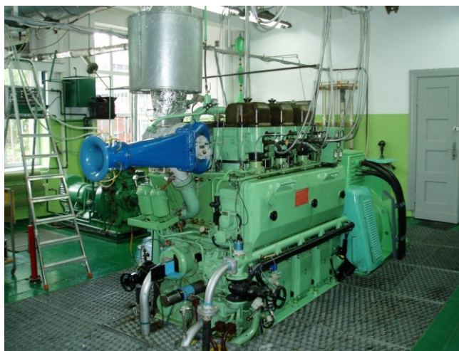
Fig. 1. Photo of the SULZER 3AL25/30 piston engine.
