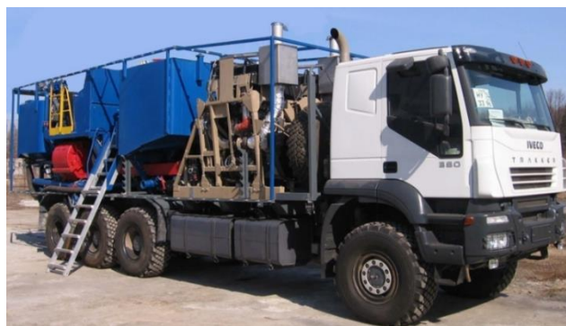
Fig. 9 Pumping facility UNBS2-600x70
