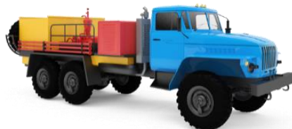
Fig. 1 Cementing truck (TSA-320)
