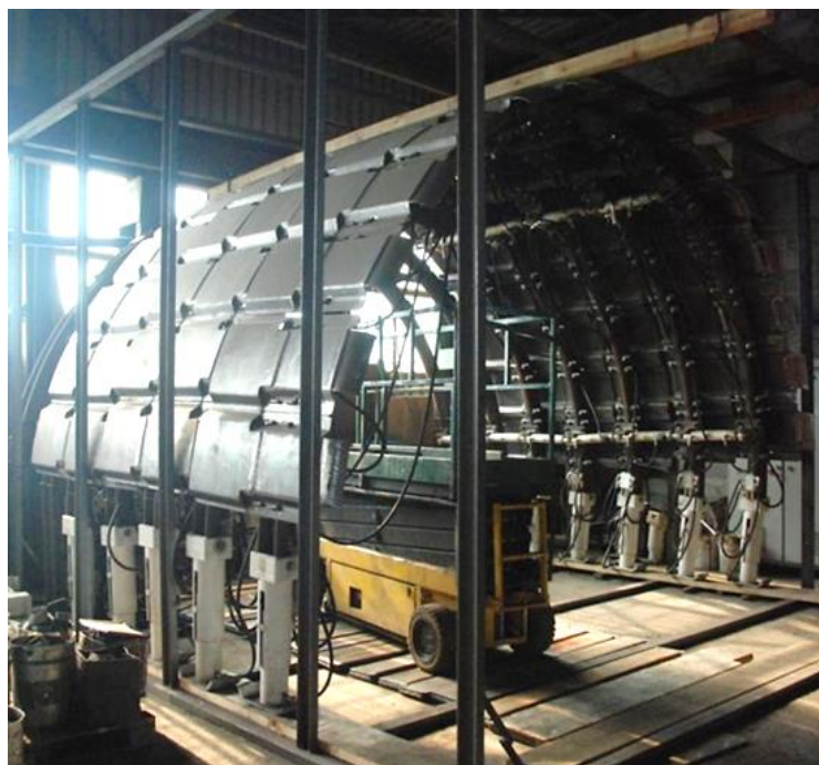
Fig. 2 View of a set of six arches of a temporary mechanized roof support
