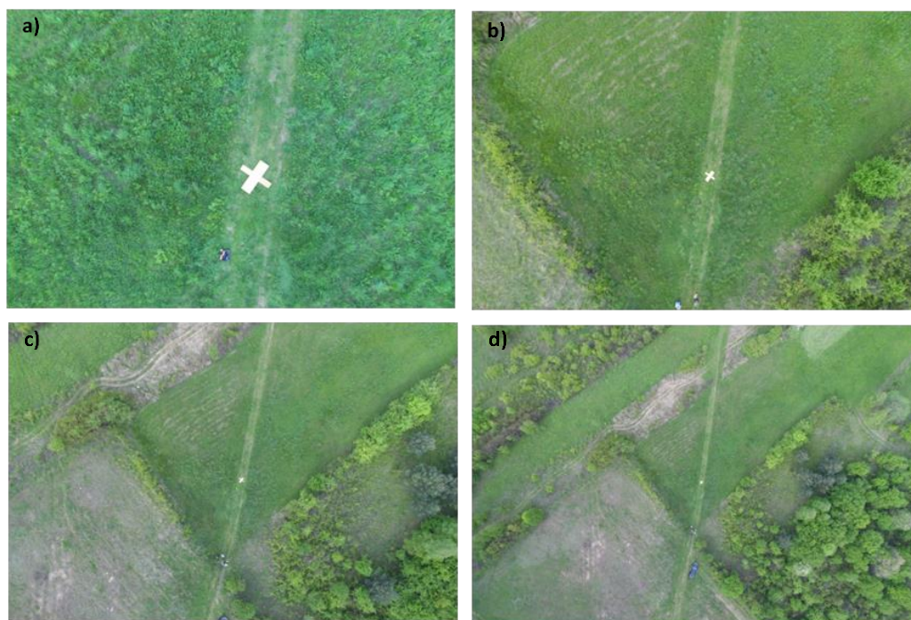
Fig. 7 Photos taken with Yuneec H520 drone with E90 camera from a height: a) 10 m, b) 30 m, c) 60 m, d) 100 m
