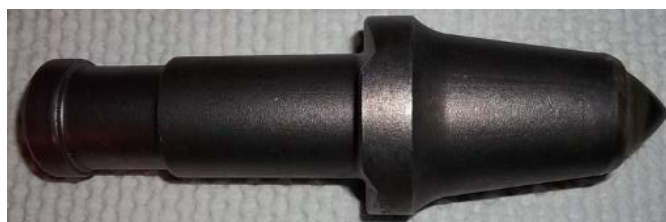
Fig. 1 Tangential-rotary knife used in the head of POU-BW/01-WAP device
