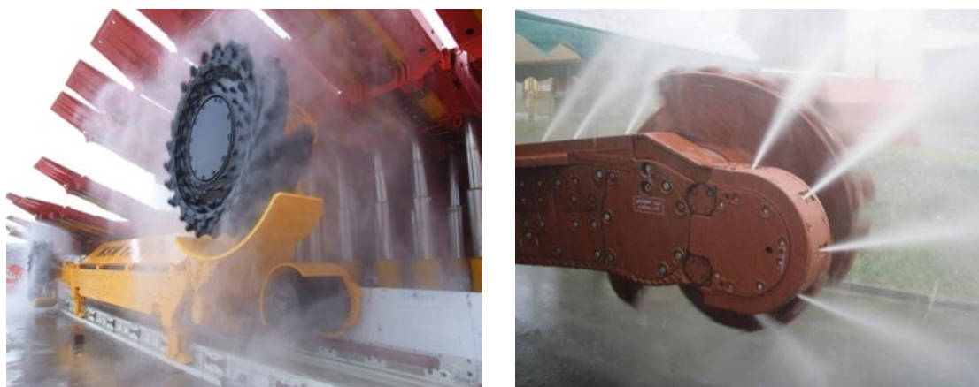
Fig. 3 System of external spraying for a longwall shearer
