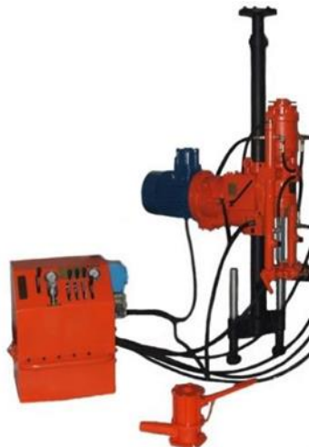
Fig. 5 WMD-150 small size drill rig
