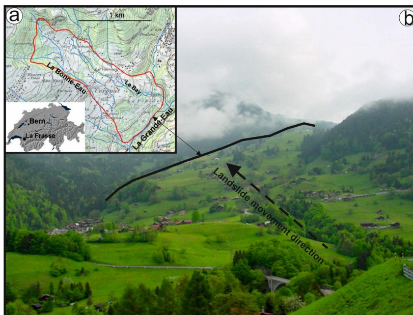
Fig. 6 a) The location (Tacher et al., 2005) b) general view of Lafrasse Landslide Sion-Switzerland
