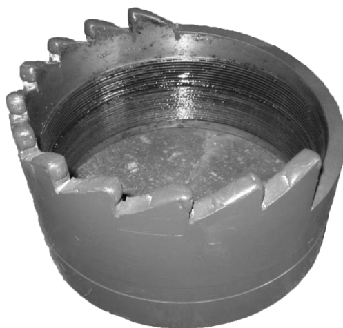
Fig. 7 General view of junk mill with hardfaced and painted working surface
