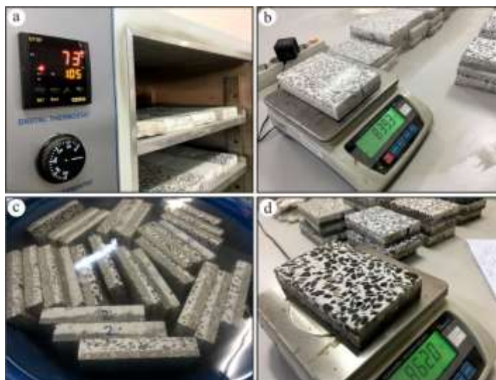
Fig. 6 Determination of unit volume weight and water absorption values of the tiles.
