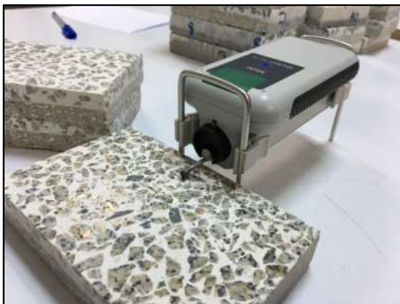
Fig. 10 Surface roughness measurement
