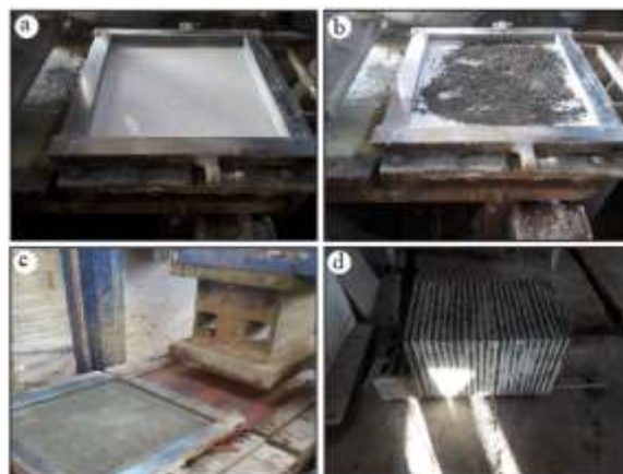
Fig. 3 Preparation of tile samples a) Pouring the top layer mortar, b) Pouring the substrate layer mortar, c) Hydraulic press, d) Waiting for the samples to freeze
