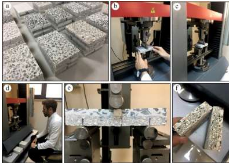
Fig. 7 Determination of bending resistance of tile samples. a) Test samples, b, c, d) Placing the sample into the device and performing the experiment, e, f) Fracture
