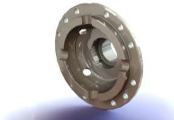
Fig. 2 3D-model of part 130-2403020-2 named “Flange half of differential case”
