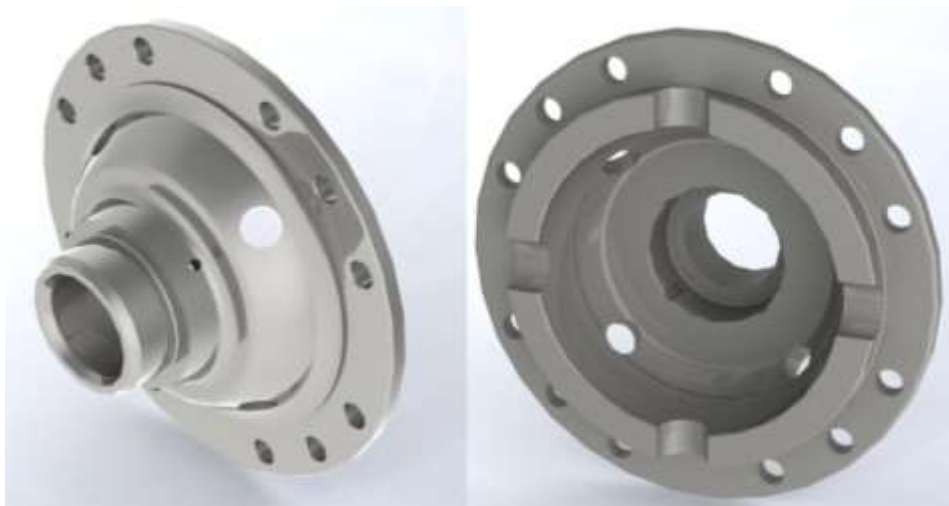
Fig. 6a The results of modelling of part “Flange half of differential case”, made of steel MSt.6: general view of the model
