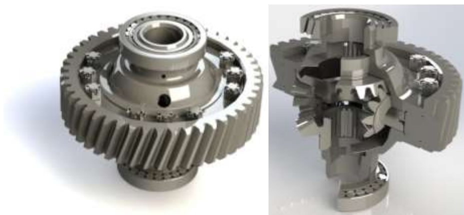
Fig. 1 3D-model of a differential of rear axle 130-2403010 in assembly and in section
