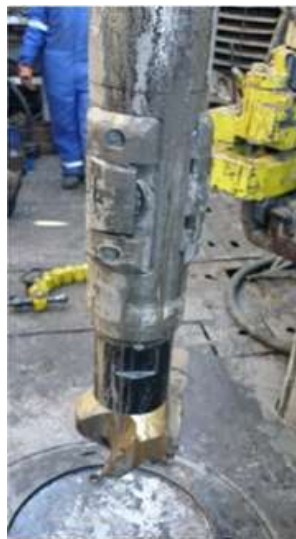
Fig. 6 Rotary steerable system before launching into the well
