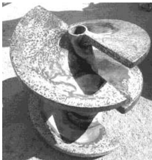
Fig. 7 General view of multi-section extruder-screw for pressing ceramic building materials (CBM) after hardfacing
