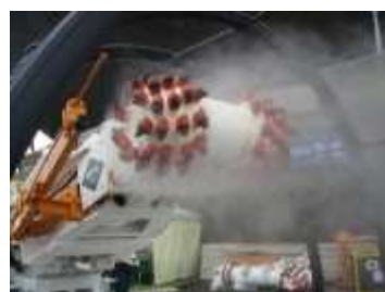
Fig. 11 Air-and-water curtain installed on the R-130 roadheader
