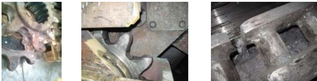
Fig. 6 Wear of teeth in wheels and toothed bars
