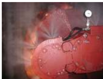
Fig. 9 KSW-460 NE shearer during the tests of extinguishing an ignition of combustible dust mixture, initiated by explosives, with use of air-and water spraying system
