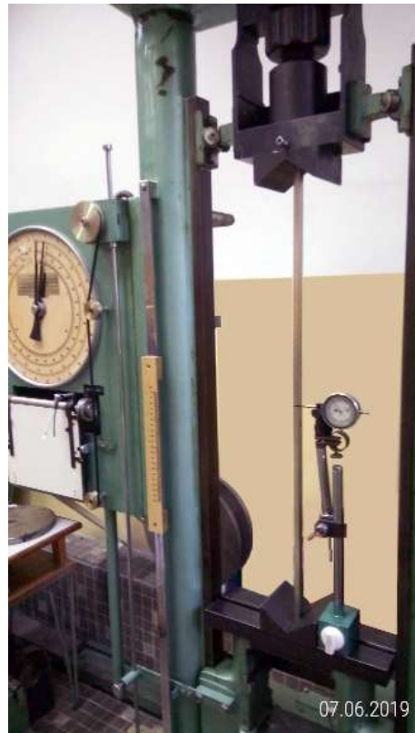
Fig. 7 A bar examined for buckling on a strength tester FM 2500
