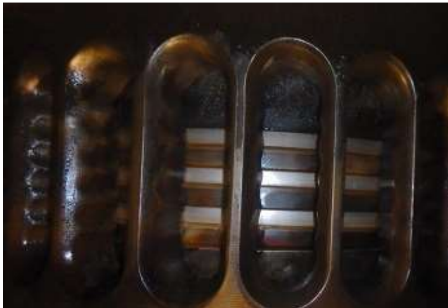
Fig. 17 Feed rate of 0.6 g/kWh after 72 hours operation with CLO BN 100
