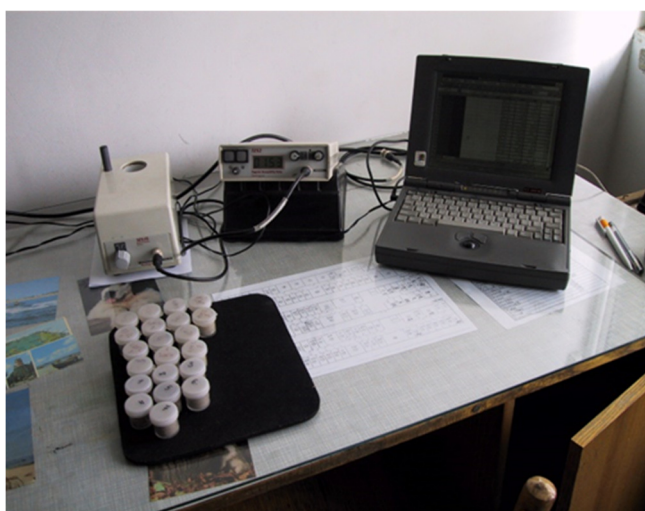
Fig. 3 Laboratory system with a MS2B Bartington device for magnetic susceptibility measurements
