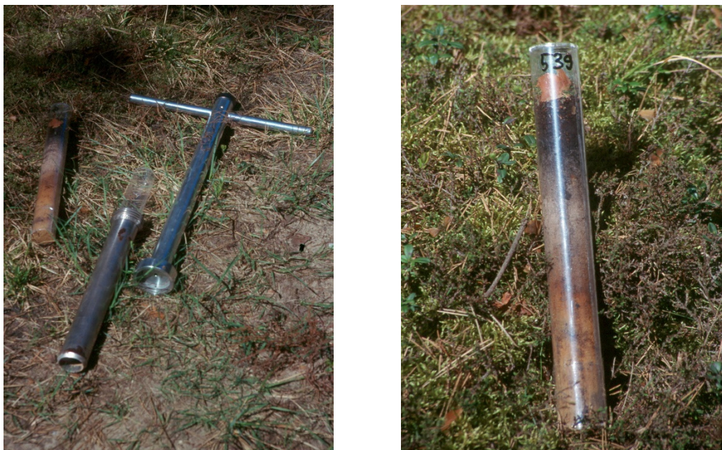
Fig. 2 a) Humax sampler, b) 30 cm length soil profile taken using Humax sampler Source: (Magiera, Zawadzki, 2006).
