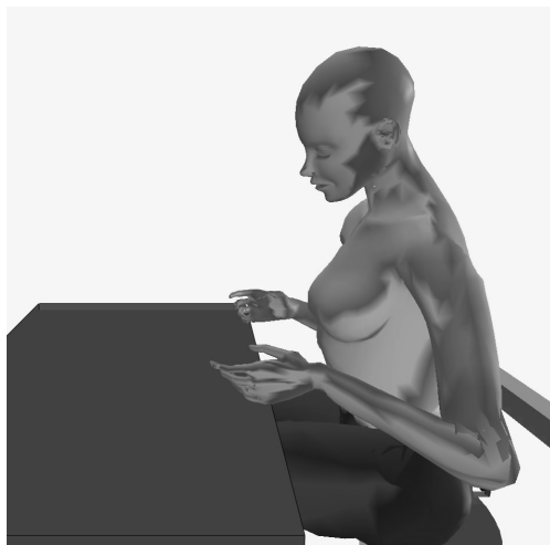
Fig. 2. Incorrect, too high position of the table top surface
