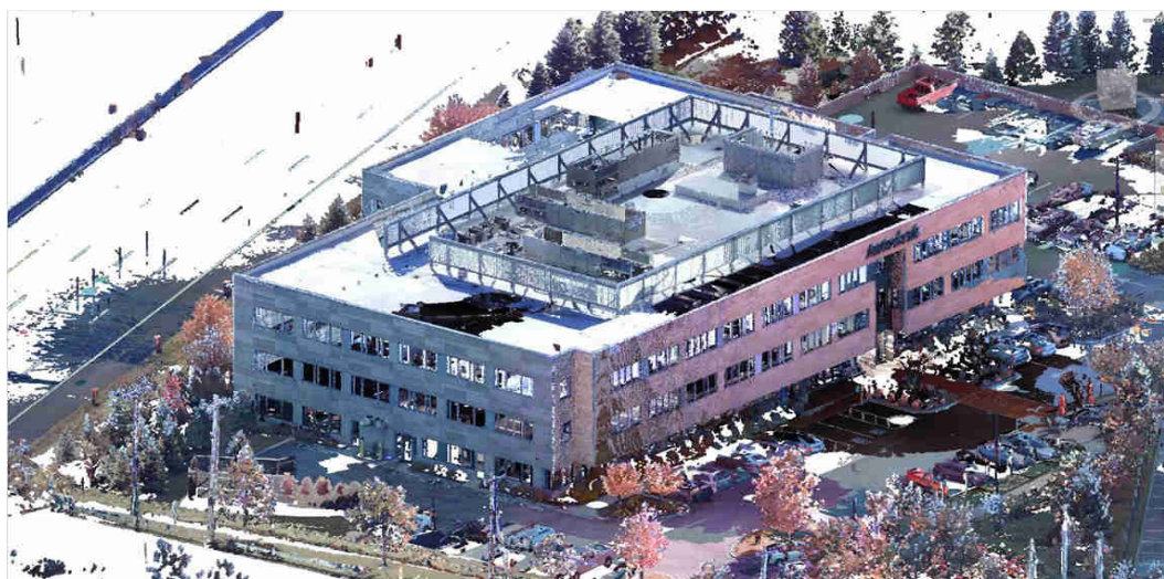
Fig. 1. Point cloud – a fragment of a scanned object
