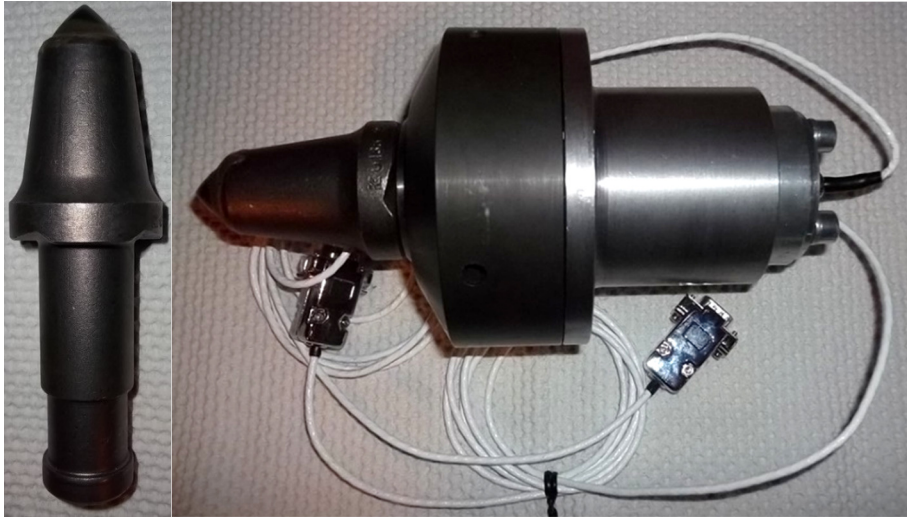
Fig. 5. The pick and measuring head with the pick installed
