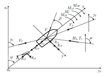
Fig. 1 The components of the total resistance of the ship (sea water flow:  $R_x$ ,  $R_y$ ,  $M_z$ ; wind:  $R_{xA}$ ,  $R_{yA}$ ,  $M_{zA}$ ; wave:  $R_{xW}$ ,  $R_{yW}$ ,  $M_{zW}$ ; rudder fin:  $R_{xR}$ ,  $R_{yR}$ ,  $M_{zR}$ ); speed V, the angle of the exchange rate  $\psi$  and drift angle  $\beta$  ship; current parameters  $V_C$ ,  $\gamma_C$ ; wind:  $V_A$ ,  $\gamma_A$ ; wave:  $H_S$ ,  $T_1$ ,  $\mu$ ; the angle of the rudder  $\delta$
