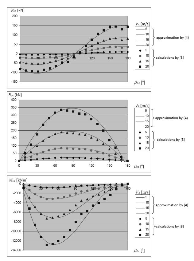
Fig. 3 The forces and moment from the wind for different wind speeds  $V_A$  - bulk carrier M1
