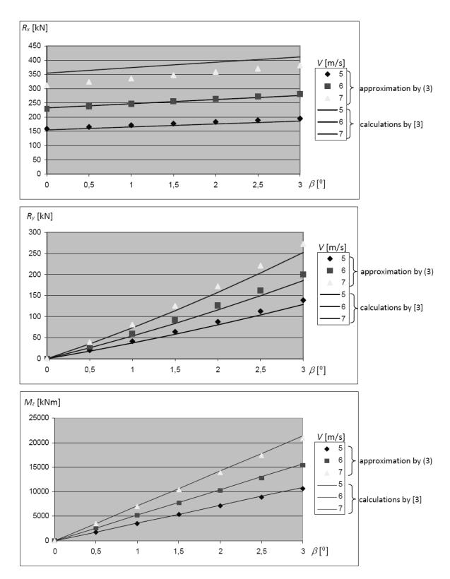
Fig. 2 The forces and moment of resistance of the ship in calm water, taking into account the angle of drift for various vessel speed V - bulk carrier M1
