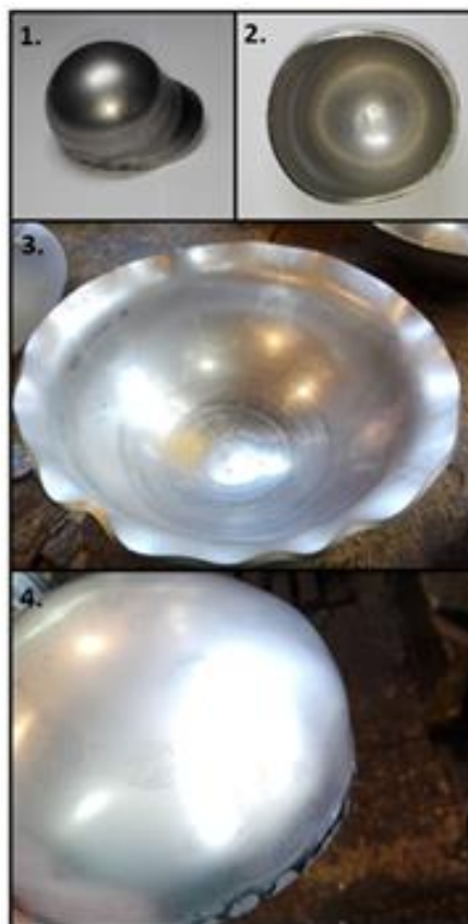
Fig. 2 Defects in stampings – 1, 3, 4 – shape defects, 2 – folding
