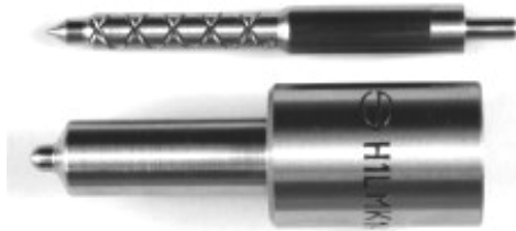
Fig. 1 Needle and body of fuel injector in a self-ignition engine with preliminary fuel treatment
