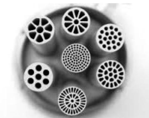
**Fig. 2 Ceramic tubular membranes with different number of channels**
