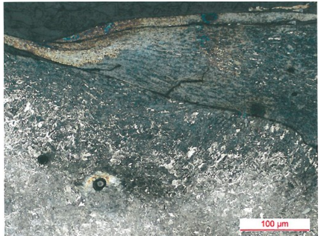
Fig. 4 The depth of cracks in sample 7A of the material collected from the bottom part of the track groove
