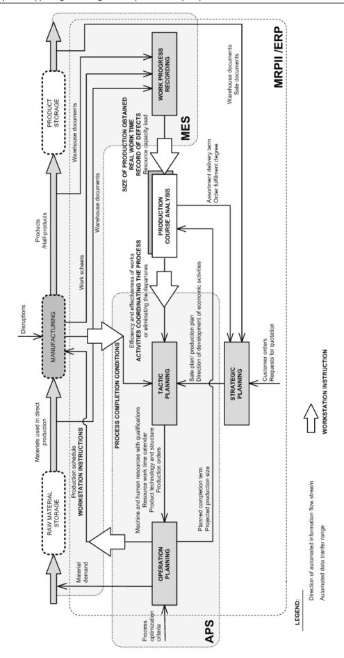
Fig. 3 The automation of information flow stream in a production control system
