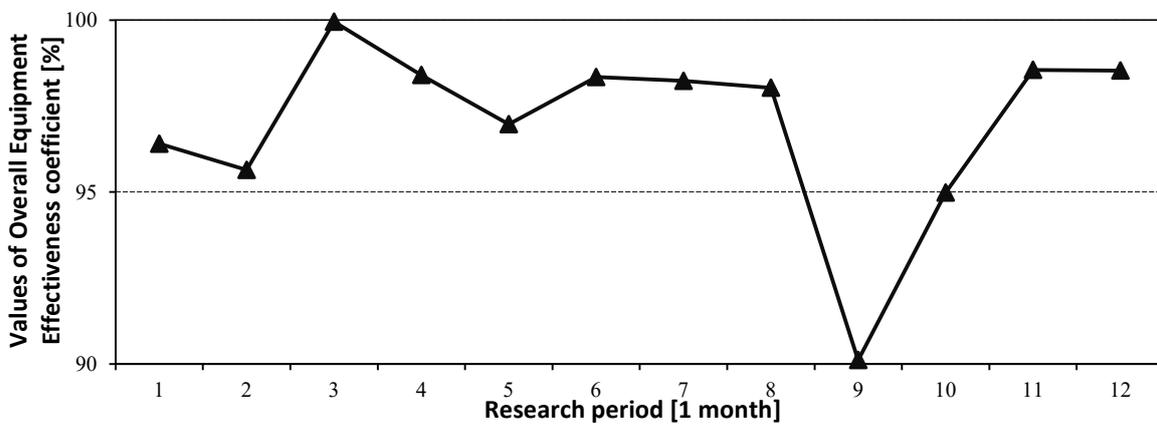
**Fig.9.4** Graphic interpretation of the Overall Equipment Effectiveness coefficient for wave soldering machine
