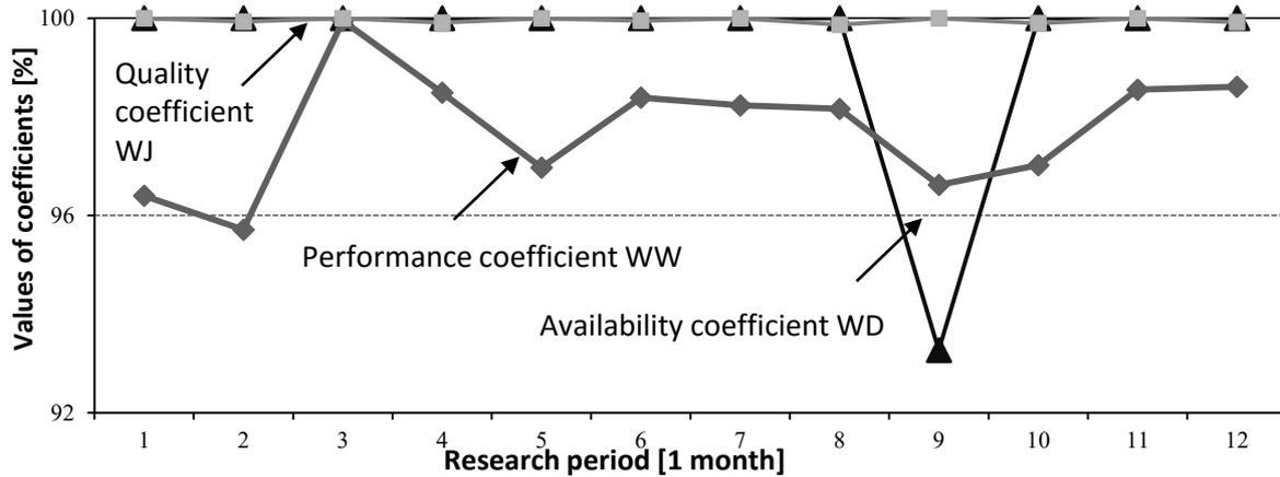
**Fig. 9.3** Graphic interpretation of the availability coefficient, performance coefficient and quality coefficient in research period for wave soldering machine
