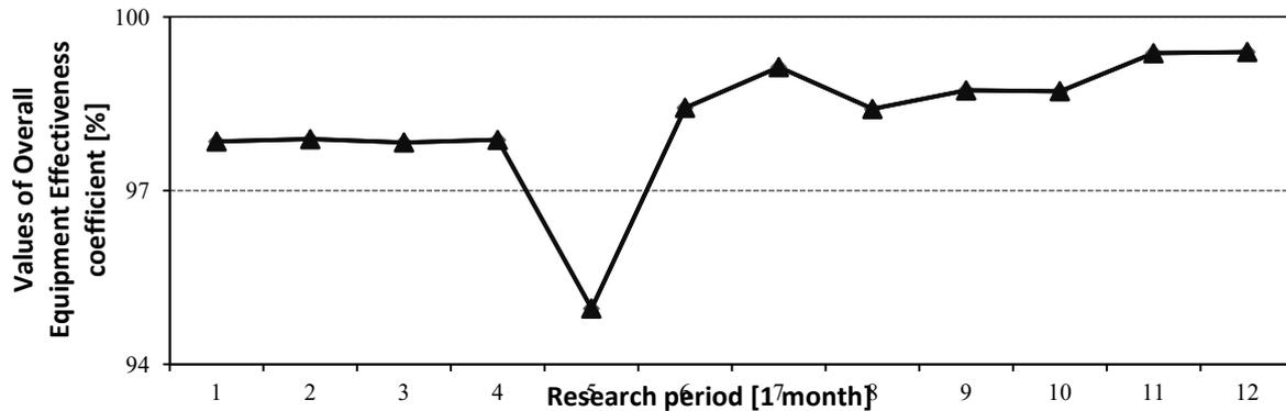
**Fig. 9.2 Graphic interpretation of the Overall Equipment Effectiveness coefficient for surface mount assembly machine**
