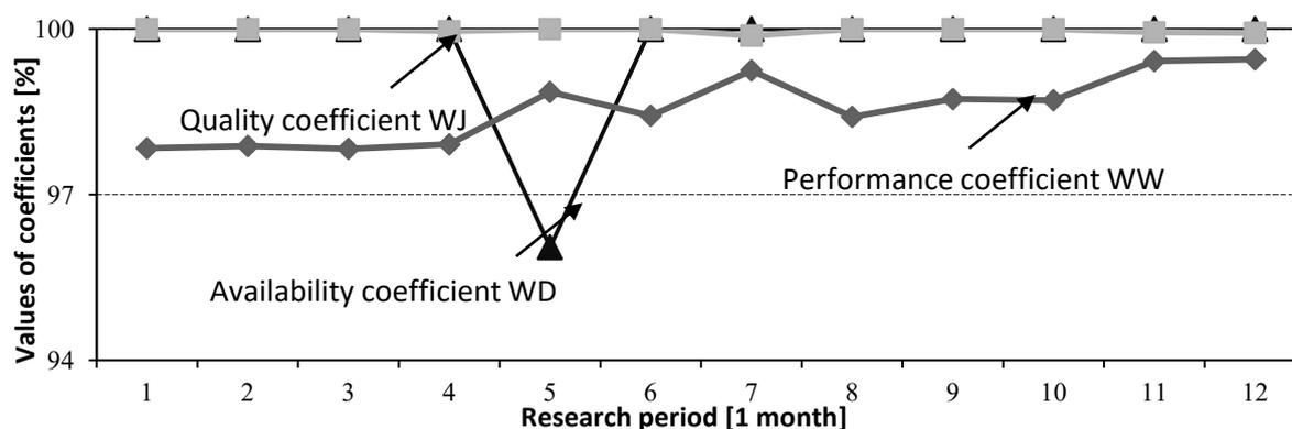
**Fig. 9.1 Graphic interpretation of the availability coefficient, performance coefficient and quality coefficient in research period for surface mount assembly machine**
