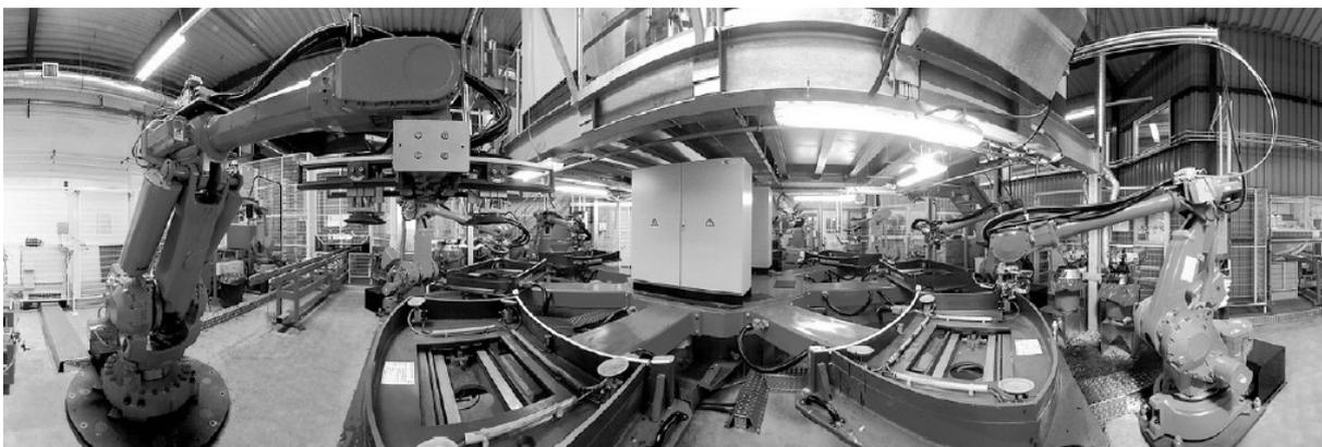
**Fig. 11.1 Rotary table where extrusion process is performed**
