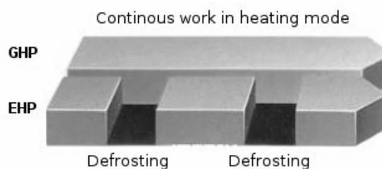
**Fig. 9.4 Difference in continuity of operation for gas (GHP) and electric (EHP) heat pumps in heating mode**
