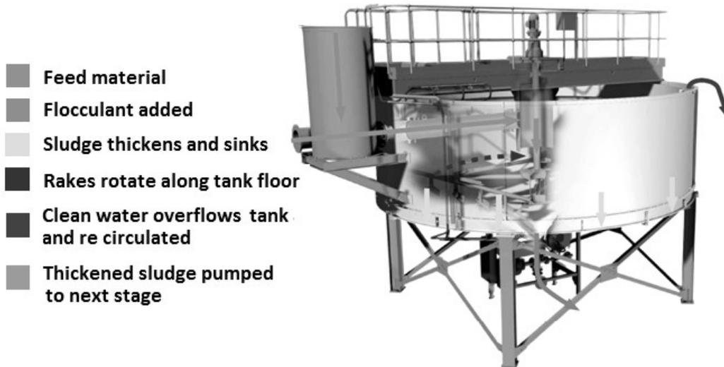
**Fig. 7.1 Scheme of radial settler tank with coagulation chamber**
