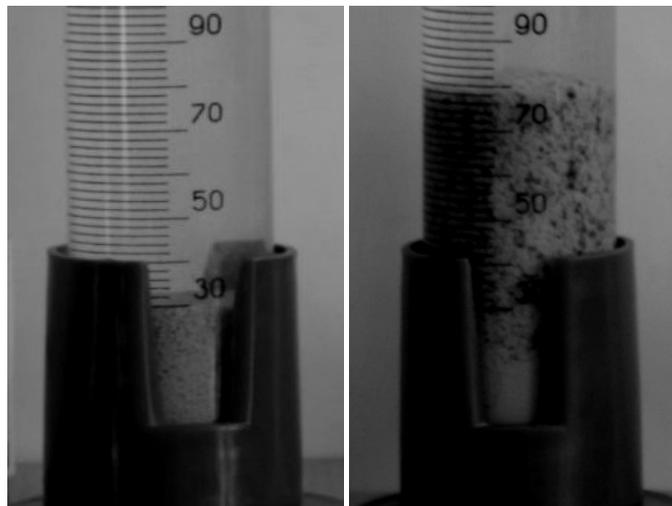
**Fig. 7.3 The character of sediment after the addition of flocculant dose concentration of 0.2% (picture left) and 0.6% (picture right) to hydromixture with mass concentration  $C_m = 9.3\%$**
