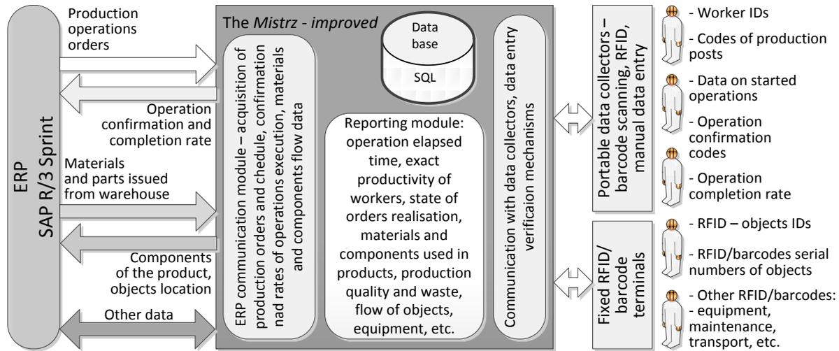
**Fig. 6.3 Proposed modifications in the data acquisition system**
