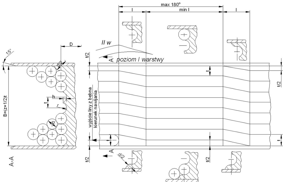
Fig. 5.9 Winding, using the synchronous LeBus method [4]
