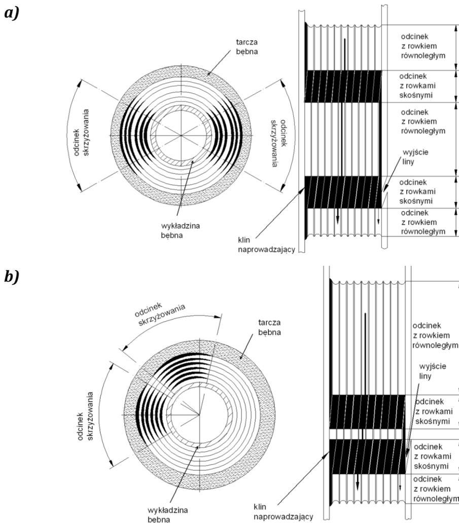
**Fig. 5.8 Schemes of multi-layer winding of ropes on the drums of LeBus method [14]:
