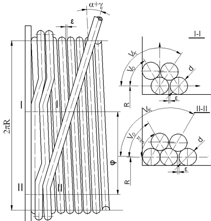
**Fig. 5.5 Diagram of the rope transition from coil to coil during multi-layer winding on cylindrical drum with helical grooves [7], I-I the first transition (the first pitch), II-II – second rope transition (the second pitch)**
