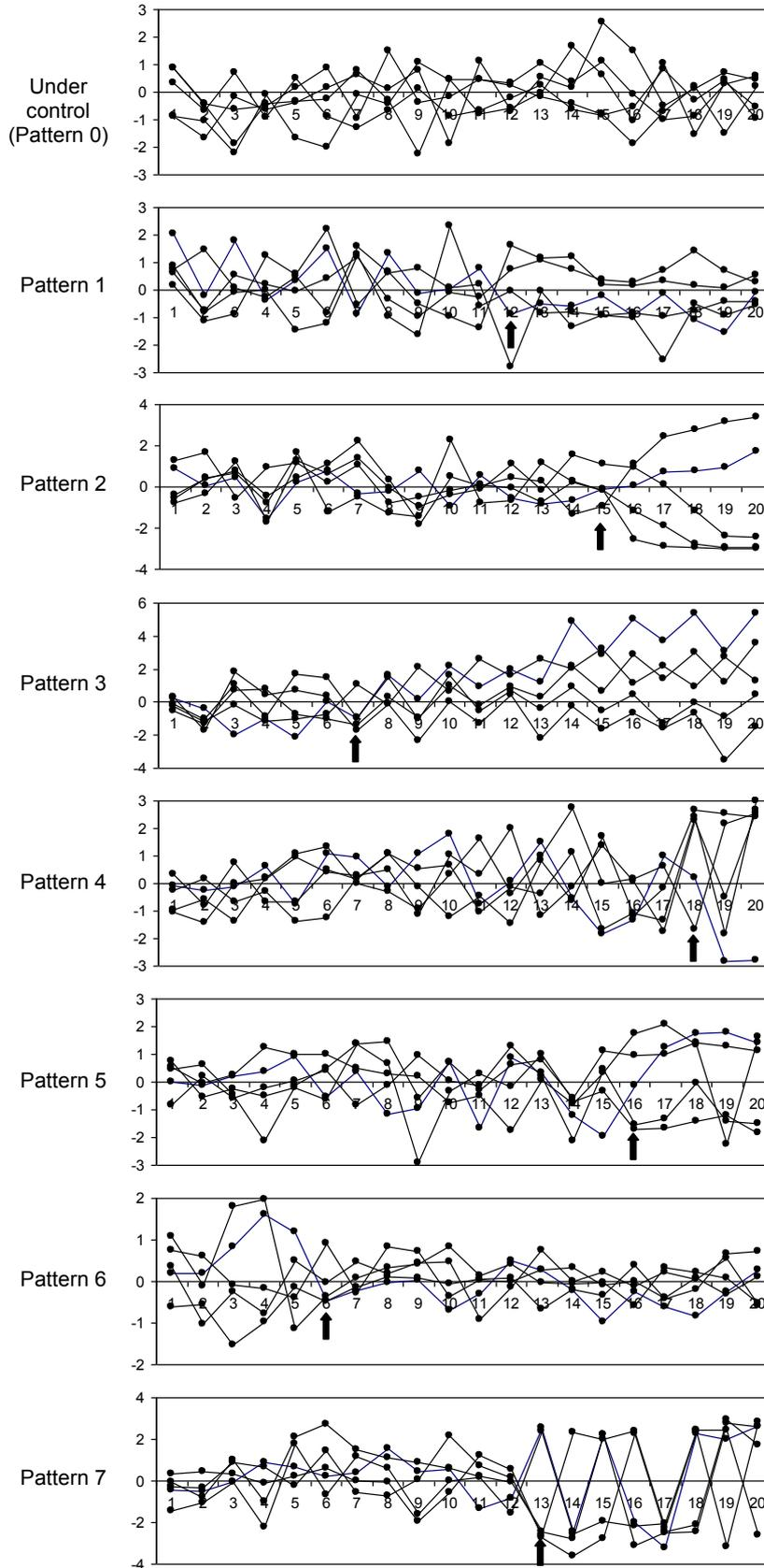
**Fig. 10.9** Examples of the records used for testing the ANNs and DTs abilities to identify the out-of-control patterns
