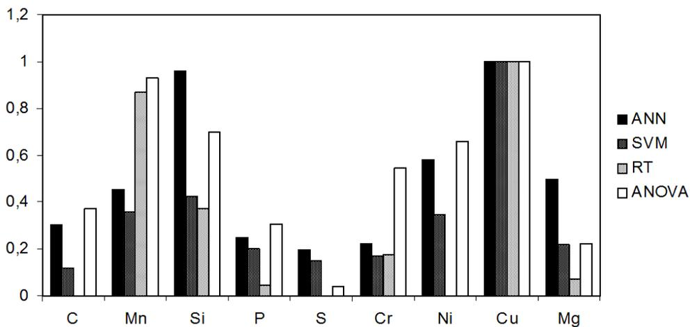
**Fig. 10.5 Relative significance factors for the industrial data set (tensile strength of ductile cast iron vs its chemical composition defined by 9 elements) obtained from regression models using various learning systems and ANOVA [18]**
