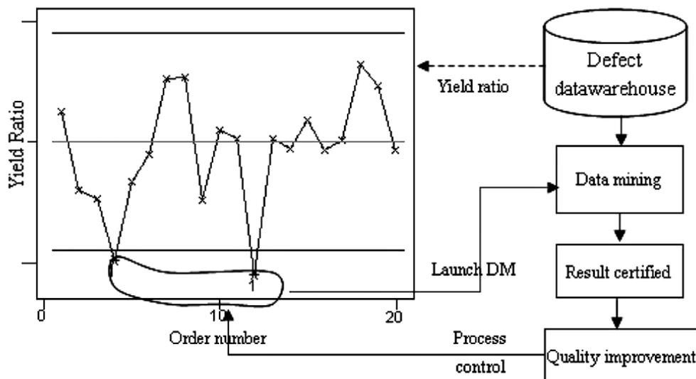
**Fig. 10.1 Scheme of continuous quality improvement system [24]**
