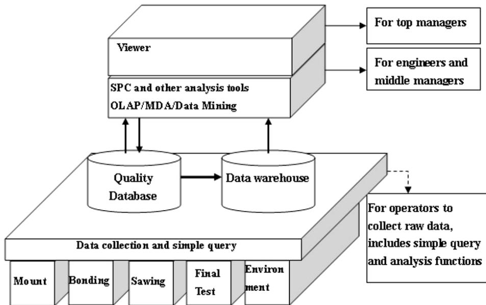
Fig. 10.2 Three-layer system infrastructure [24]
