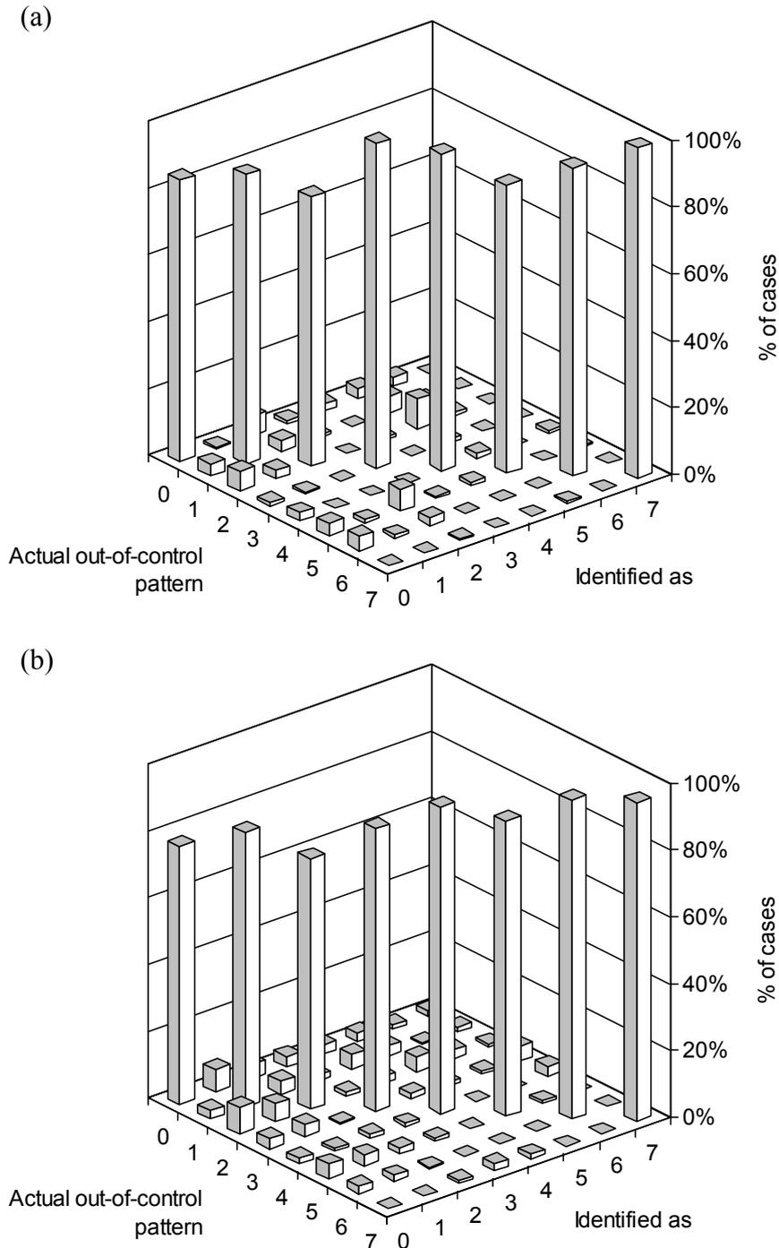
**Fig. 10.12 Distribution of correct and incorrect classification fractions obtained for the training data set including all out-of-control patterns: (a) from DTs, (b) from ANNs**
