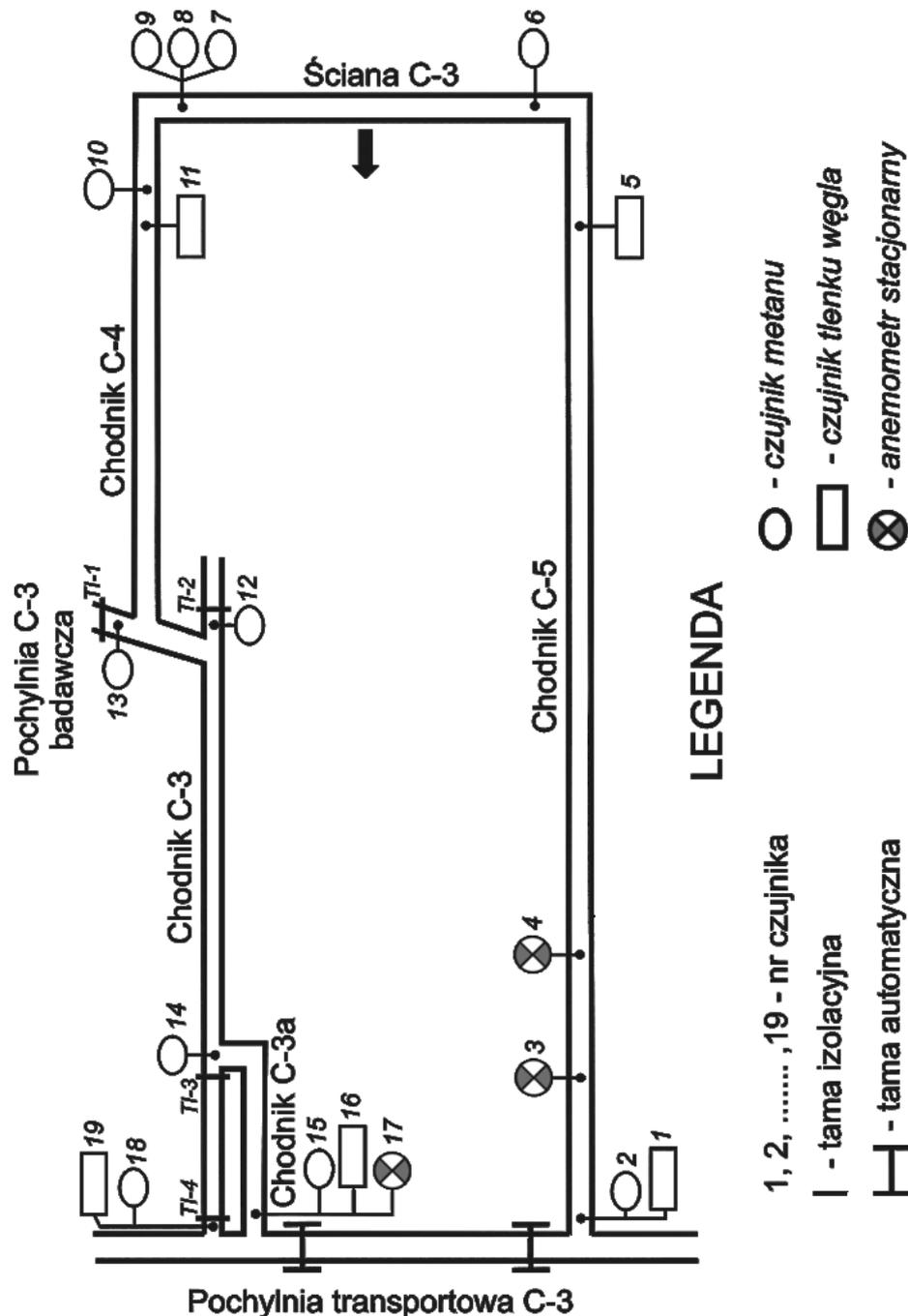
*Fig. 1.10 Example of detector's arrangement in the longwall*
