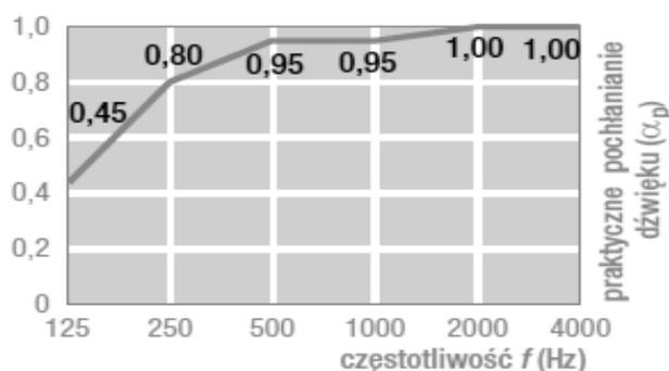
**Fig. 19.4 Graph of acoustic absorption THERMATEX Alpha Black [7]**
