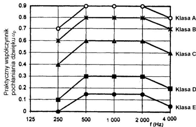
Fig. 19.2 Reference curves illustrating the absorption class [4]
