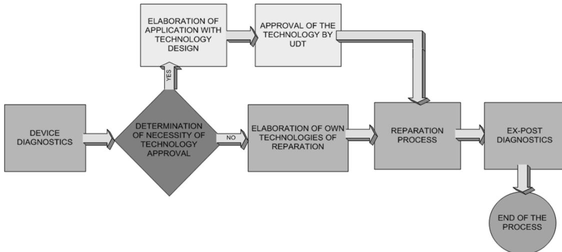
**Fig. 14.5 Algorithm of activities of a company authorised for performing reparations and modernisations of handling equipment [8]**
