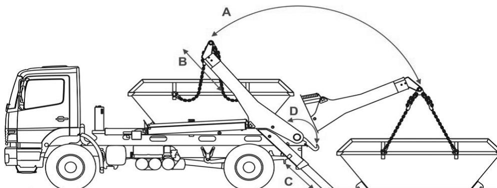
**Fig. 14.2 Working movements of a skiploader [3]:**
