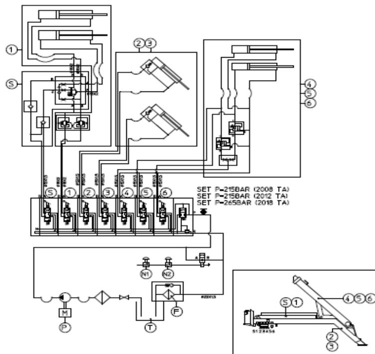
**Fig. 14.7 Hydraulic scheme of a skiploader [9]:**
